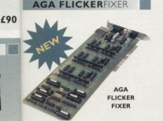
ScanDoubler II is a full 24-bit AGA Flicker Fixer for the Amiga 4000. It automatically de-interlaces all AGA screen modes and scan-doubles non-interlaced PAL/NTSC modes to allow VGA monitors to display them. Supports VGA only, S-VGA and Multiscan monitors. Pixel sharp picture, even at 1440 horizontal resolution and has a standard 15 pin VGA type connector. Comes with composite video/S-VHS outputs.
